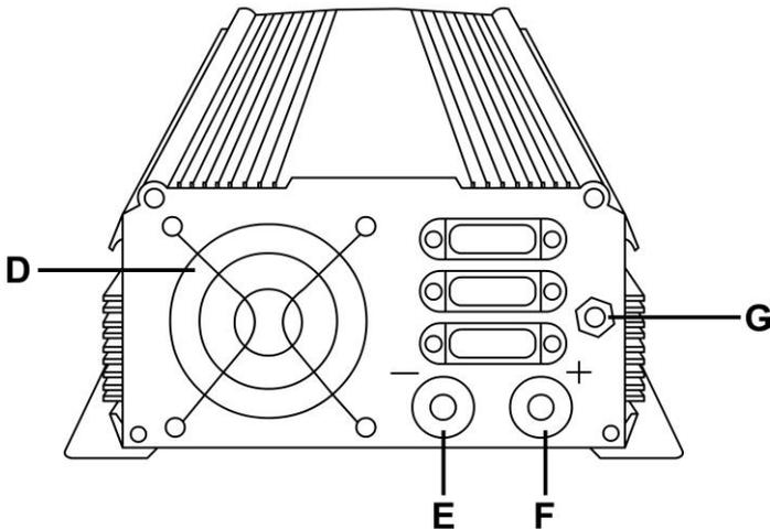
D. High-Speed Cooling Fans. When the temperature inside the inverter exceeds a preset limit, the Cooling Fan automatically turns on to cool the inverter. When the temperature reduces, the fan turns off.
