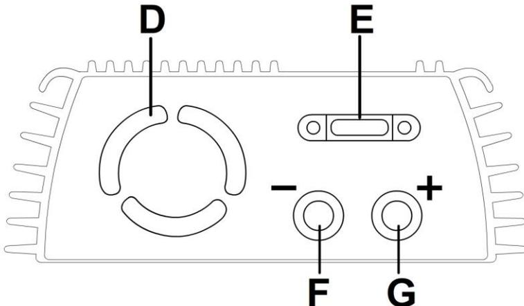
D. High-Speed Cooling Fans. When the temperature inside the inverter exceeds a preset limit, the Cooling Fan automatically turns on to cool the inverter. When the temperature reduces, the fan turns off.
